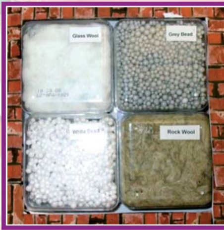
The types of cavity wall insulation used are mineral wool (glass or rock), EPS beads (white or grey), or UF foam.
