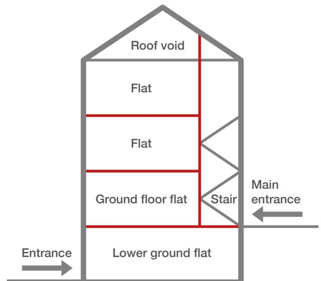
— Fire-resisting compartment wall and floor
